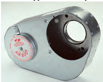
Combustion air boot: This metal boot attaches to the air intake of a power burner to provide combustion air from outdoors.
