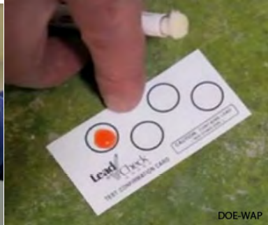
If the surface tests negative, verify the validity of the test with the calibration card provided.
